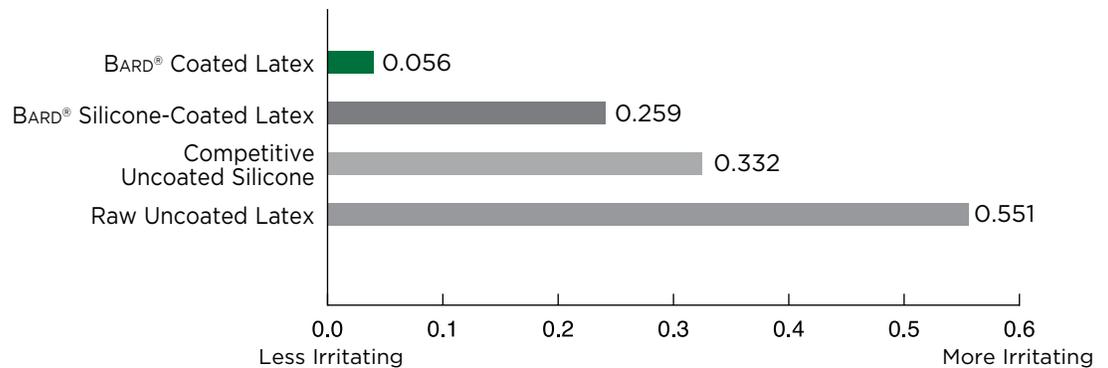
Per 24-hour hydration testing: The coefficient of friction (COF) measures the ease with which two surfaces slide against each other. A lower COF indicates less resistance, while a higher COF indicates more resistance, more friction and greater irritation.
