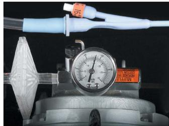
Tested competitive silicone Foley catheters cannot match Bard's funnel durability, collapsing with only -15 in. Hg.
